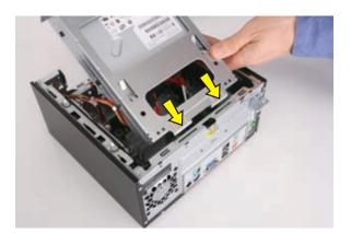
6 Replace the two optical drive cage screws.
